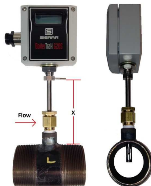
Figure 5: Meter Inserted into Pipe
