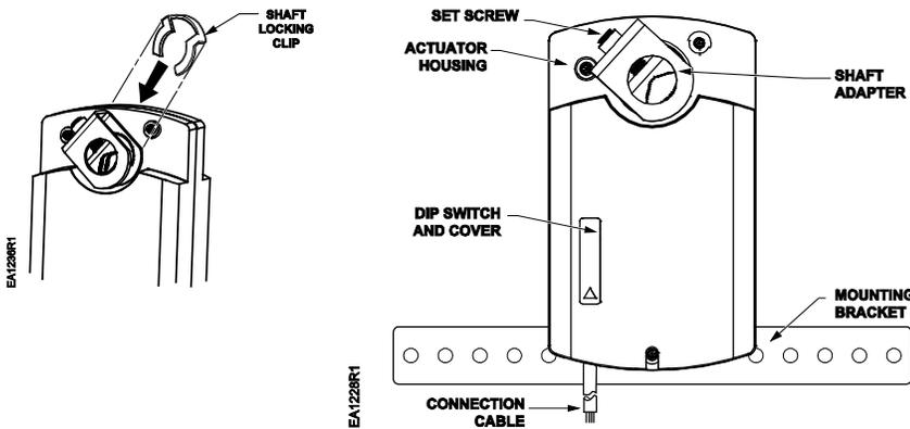
Figure 1. Components of the GQD Spring Return Actuator.
