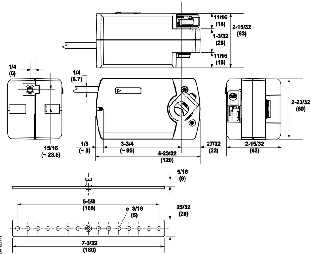
Figure 14. GQD1x1 Actuator and Mounting Bracket.
